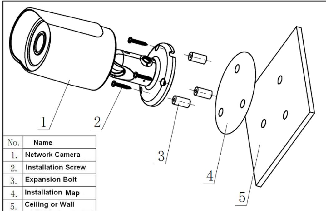
Figure 2-1 Device installation 1
