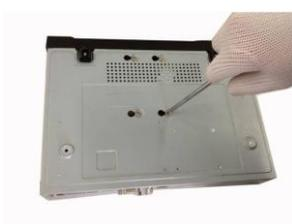
5. Fix the HDD firmly.
